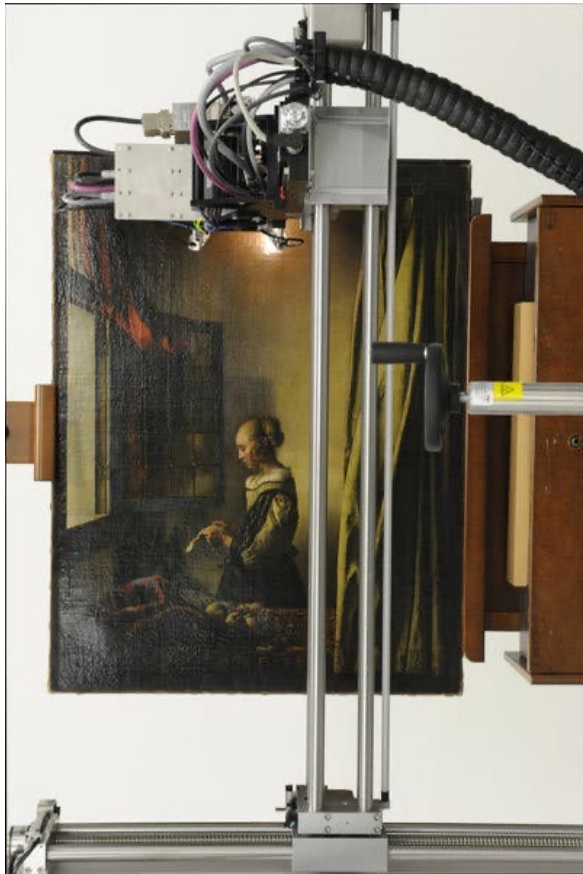
Vermeer's "Girl Reading a Letter at an Open Window" undergoing X-ray fluorescence analysis by the Dresden State Art Collections in Germany. Credit... Gemäldegalerie Alte Meister, Staatliche Kunstsammlungen Dresden; Maria Körber
