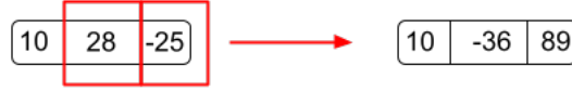
Figure 2.7: Example of mutation operator. The selected alleles, in red, are mutated to new values according the problem constraints.
