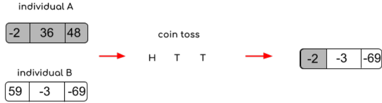
Figure 2.8: Example of crossover. The tossed coin is unbiased. So the probability to get head or tail is the same.
