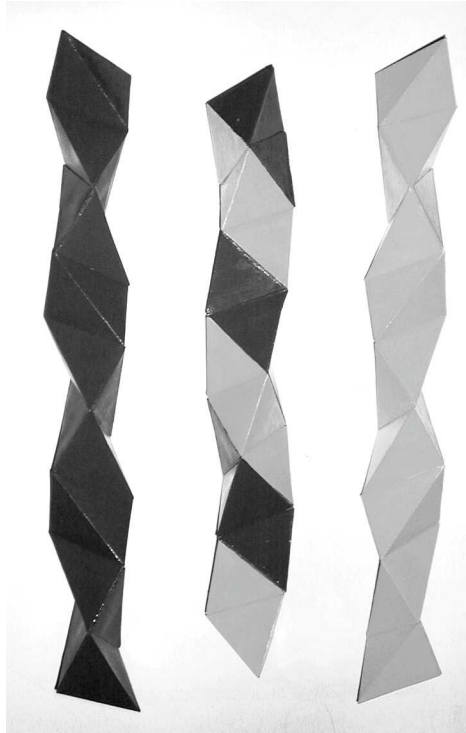
Figure 6: The picture in right hand side corresponds to a configuration with two left handed helices. The central picture and the left hand side one have three and two right handed helices on their structures, respectively.
